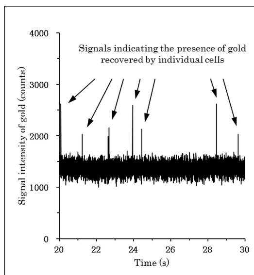
An example of analytical results of the gold-recovered *G. sulphuraria* cells from metal wastewater by using NMIJ originally-developed single-cell elemental analysis system.
