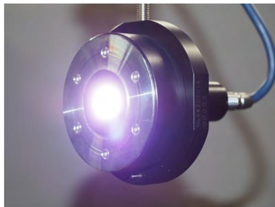
Photograph of the standard LED for  $2\pi$  TSRF
