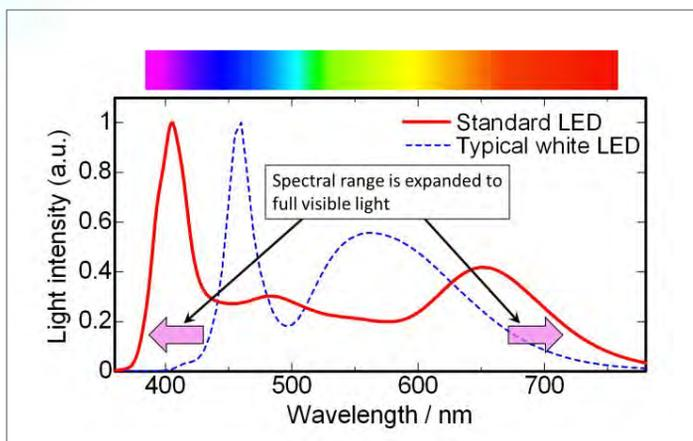
Spectra of the developed standard LED and a typical white LED
