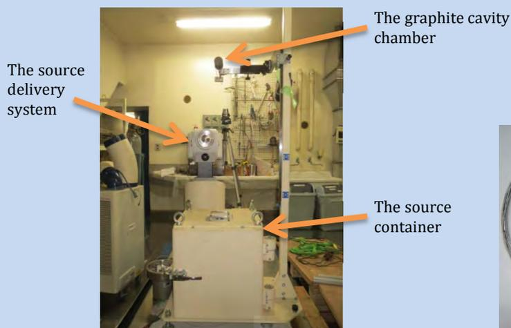
The experimental setup for the measurement of dose for the Ir-192 brachytherapy source
