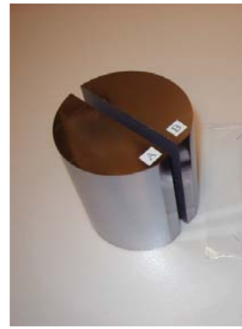
Photo 2. FZ-silicon ingot (φ5 inch x 130 mm)
